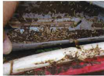
Cable inhabited by termites within.
