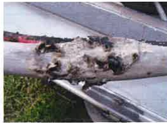
Burn marks of electric leakage caused by termites.
