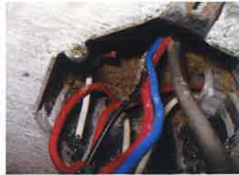
Burn marks of electric leakage caused by termites.
